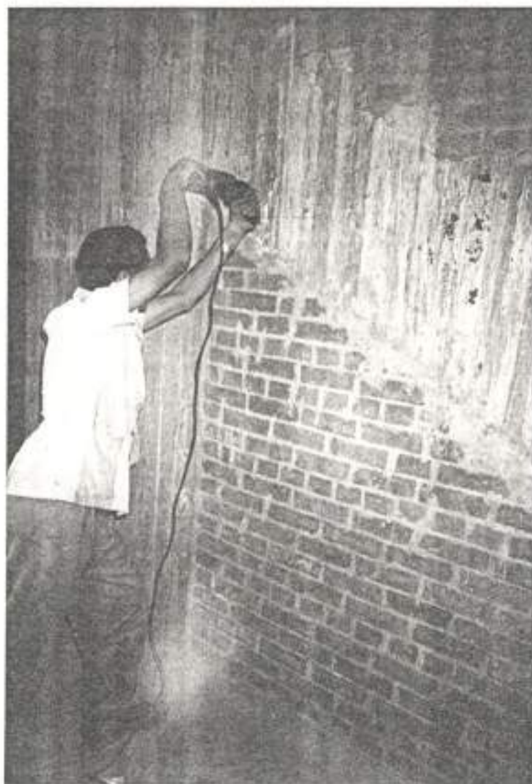
Fig. 8. In-situ setting of the air permeability test (Air Permeameter).
